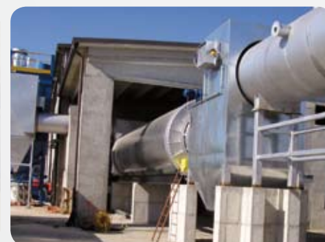
Essiccatore 6 ton/h 6 t/h chips dryer
